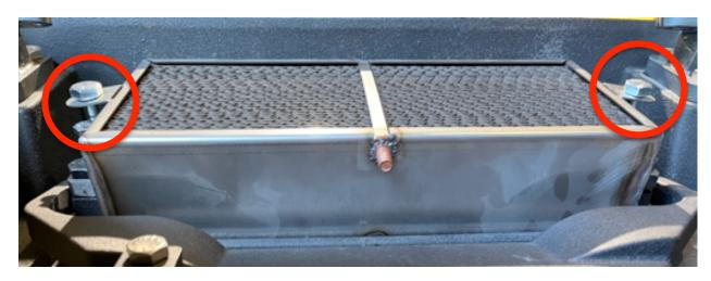
3. Re-install the Combustor Heat Shield with the included 7/16" hex nut. The curled front tabs on the combustor heat shield should rest on the top, front-facing edge of the catalyst.
