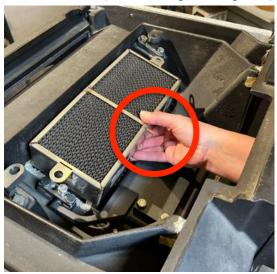
2. Apply anti-seize compound to and insert the new 5/16"-18 x 1.5" retaining bolts through the bolt tabs on the catalytic combustor, down into the corresponding holes on the combustor pan below. Using a 1/2" wrench or socket, tighten the bolts enough to create a seal between the catalytic combustor and the combustor gasket. These don't need to be over-tightened, just enough to pull the tabs on the catalytic combustor downward (see photo below).
