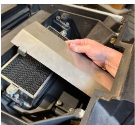
6. Remove retaining bolts (if installed) with a ½" socket or wrench from tabs on both sides
