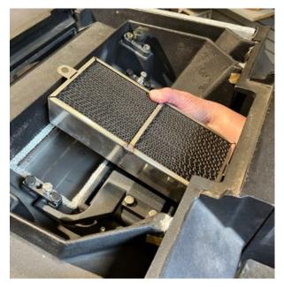
8. Inspect the under combustor gasket and replace if needed- a good seal under the catalytic combustor is critical to proper performance and efficiency. See our website (www.woodstove.com) or call us at 800-866-4344 to order a new under combustor gasket kit, which includes a proper length of gasket and the gasket glue to install it.
