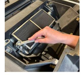
7. Lifting up and rotating 90 degrees, remove the original catalytic combustor through the open block-off collar. **Note:** your existing catalytic combustor may look different than your new one. Some older catalysts included two cast iron frames, top and bottom, which encased the catalytic element (constructed of either ceramic or steel material). Your new catalytic combustor will not utilize these frames and they may be discarded.
